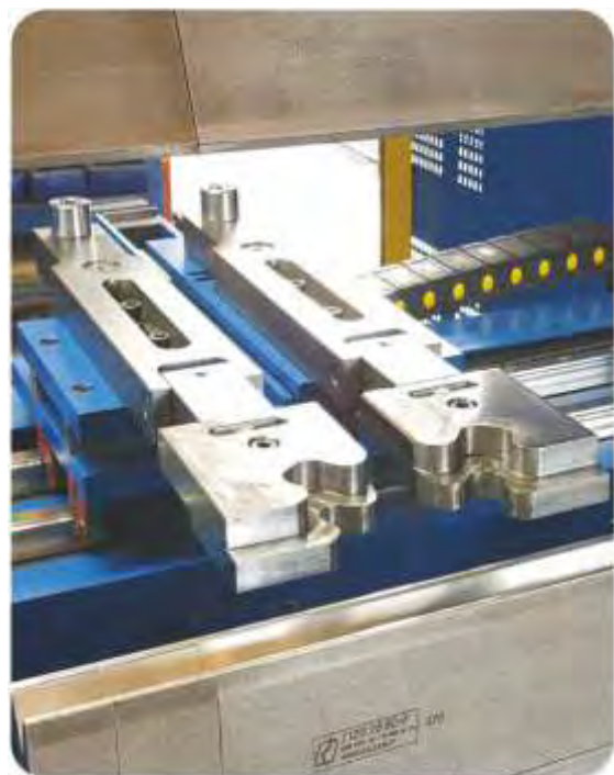
Specially designed finger stops offering high accuracy and maximum flexibility even in conical bends. Maximum stop position 1200mm
