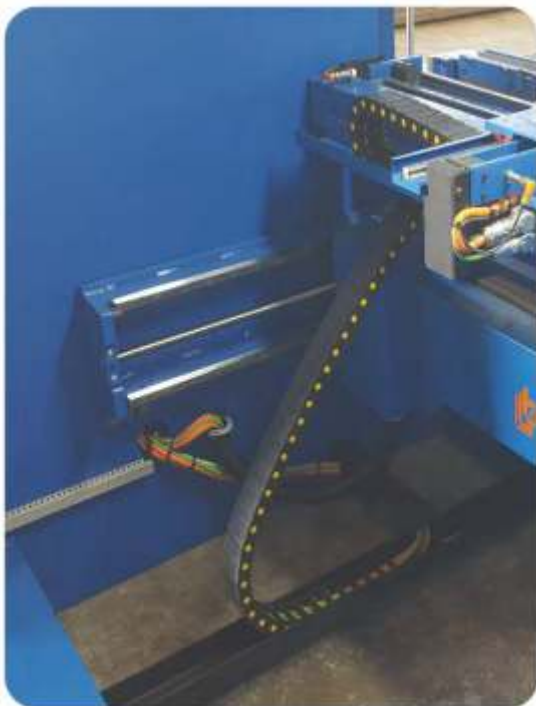
Back gauge driven through ball screw and double linear guides on every axis.
