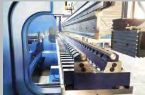
Special, heavy-duty, adjustable die, V=25 - 400mm
