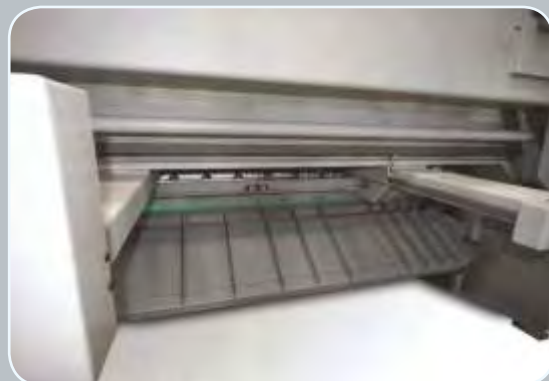
Position 3: The RSS moves even further while inclining so that the sheet-metal moves out of the machine.
